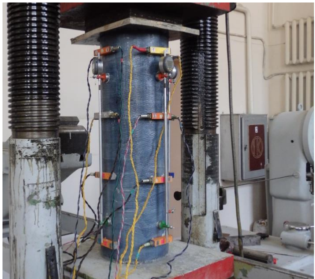
Fig. 3. Reinforced concrete specimens during static testing
