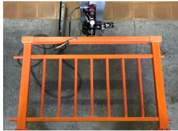
Fig. 6. Sample of the railing during static tests
