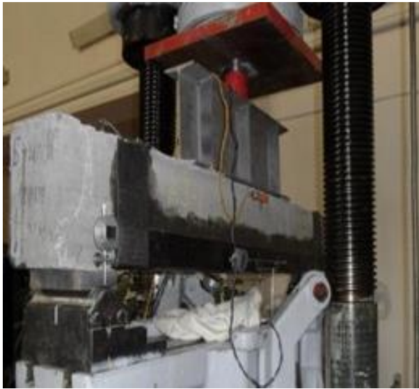
Fig. 3. Reinforced concrete specimens during static testing
