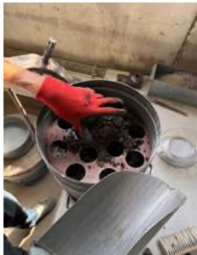
Fig. 2. Determination of the particle size distribution of milled asphalt concrete
