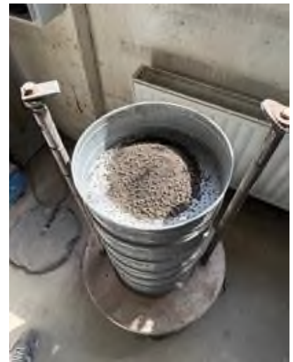
Fig. 2. Determination of the particle size distribution of milled asphalt concrete
