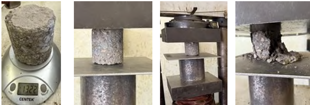
Fig. 7. Compressive strength test of core samples
