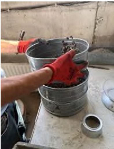
Fig. 2. Determination of the particle size distribution of milled asphalt concrete
