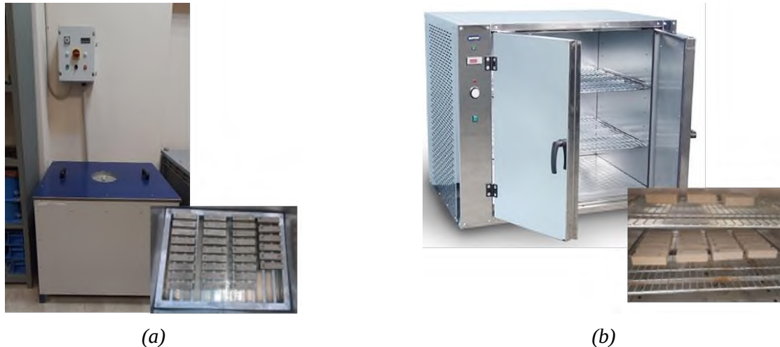
Fig. 3. Humidity test chamber (a), drying oven (b), and the specimen
