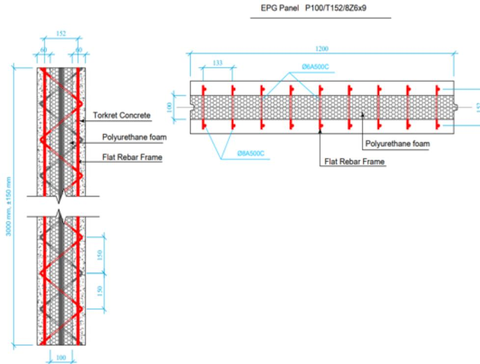
**Fig. 1.** Transverse and longitudinal sections of three-layer sound - and thermal insulating panels
