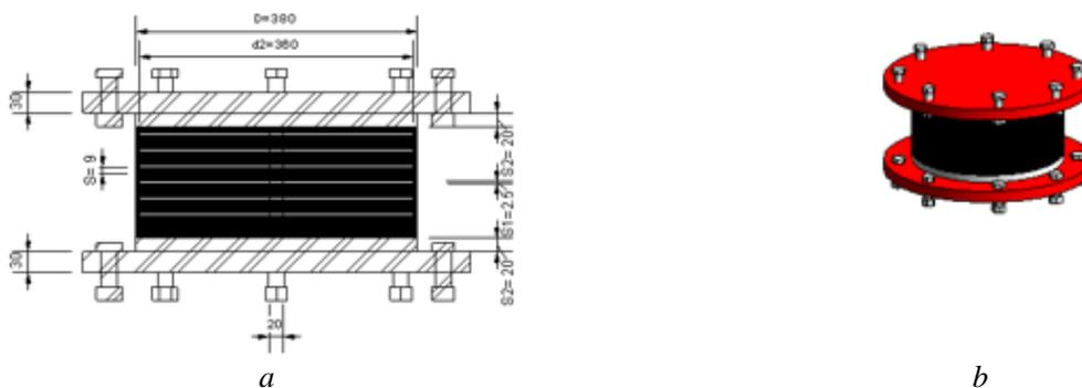
**Fig. 1.** RMLSIS used in RA, mm. a - geometric appearance, b - three-dimensional appearance
