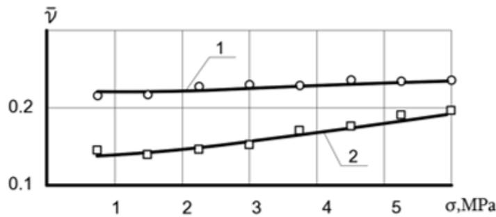
**Fig. 5.** Curves of the dependence of the coefficient of transverse deformations of soil cement samples on strength ( $\tau = 28$  days - curve 1,  $\tau = 90$  days - curves 2)
