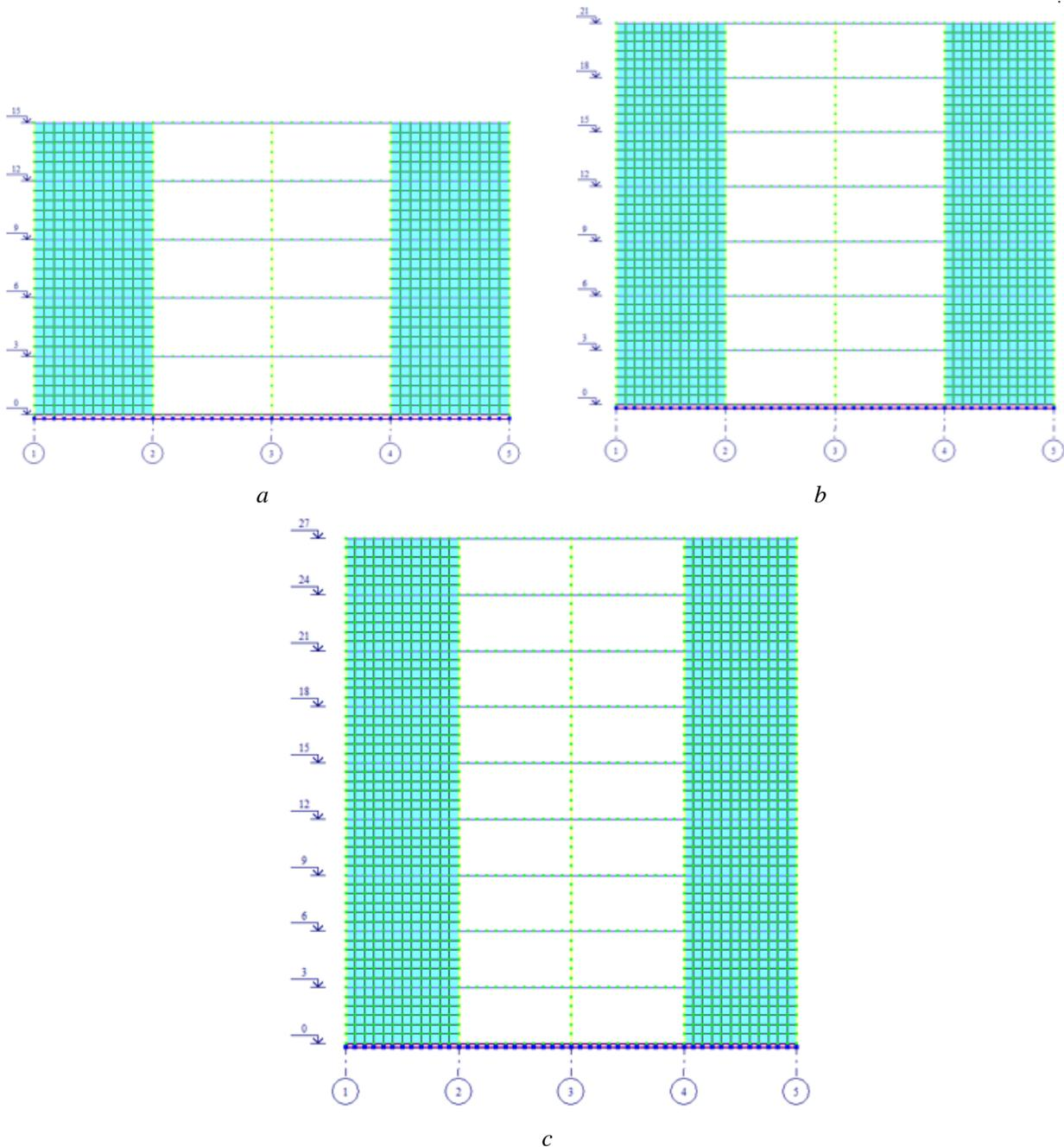
**Fig. 2.** Five-story (a), seven-story (b) and nine-story (c) building sections with "D" axis
