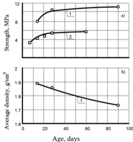
**Fig. 1.** Curves of the dependence of the strength value (a, curve 1), the average density (b, curve 1) of the soil cement based on white soils of carbonate composition and the strength (a, curve 2) of the soil cement based on clay soils on the age of the material
