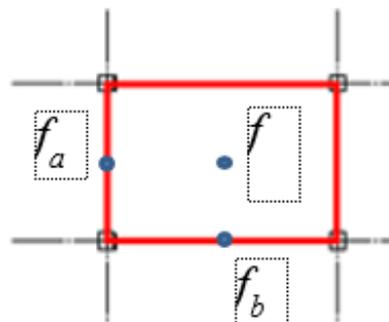
Fig.2. Characteristic points of the central cell:  $f$  - deflection in the center of the cell,  $f_a$  - deflection in the center of the smaller side of the cell,  $f_b$  - deflection in the center of the larger side of the cell
