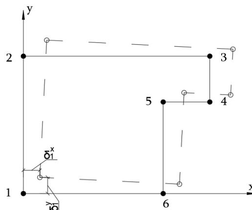
**Fig. 4.** Calculation scheme of displacement of the building formed as a result of torsion,  $\delta_1^x, \delta_1^y$  – displacement in x and y directions in point 1
