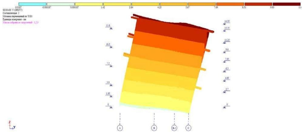
**Fig. 6.** Analytical image of floor movements from seismic horizontal load in the direction of *Y*
