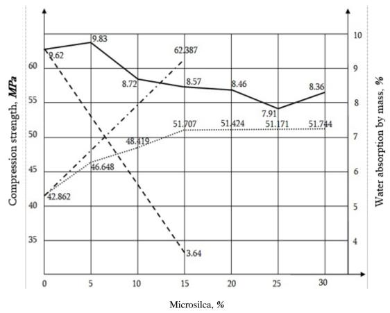
...... the limit of the compression strength depending on the quantity of microsilica,
