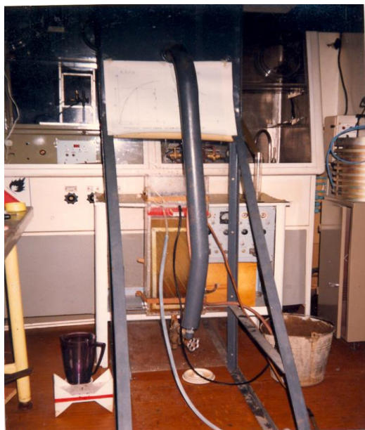
Fig. 2. Laboratory unit of a thin-layer settling tank (rectangular section)
