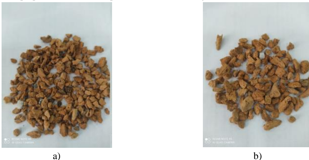
Fig. 1. Sizes of Irind mine pumice grains. a) 1.5 to 2.0 mm, b) 2.5 to 5.0 mm
