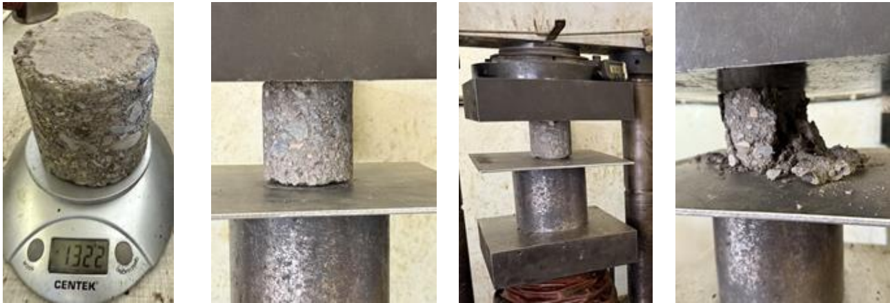
Fig. 7. Compressive strength test of core samples
