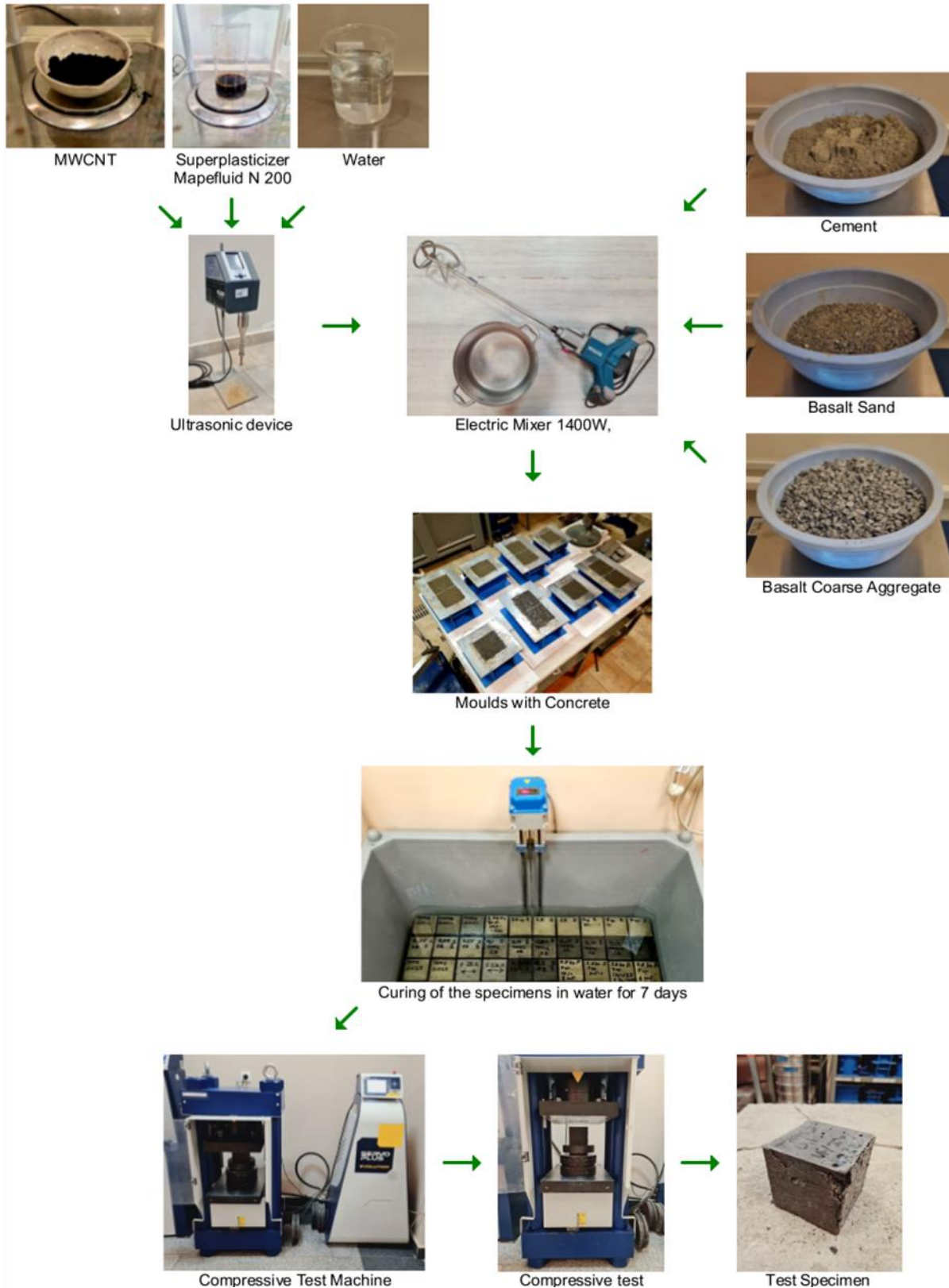
Fig. 2. Sample preparation steps, curing and testing processes
