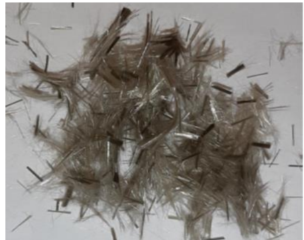
Fig. 1. Dispersed basalt fibers for cement mortar reinforcement
